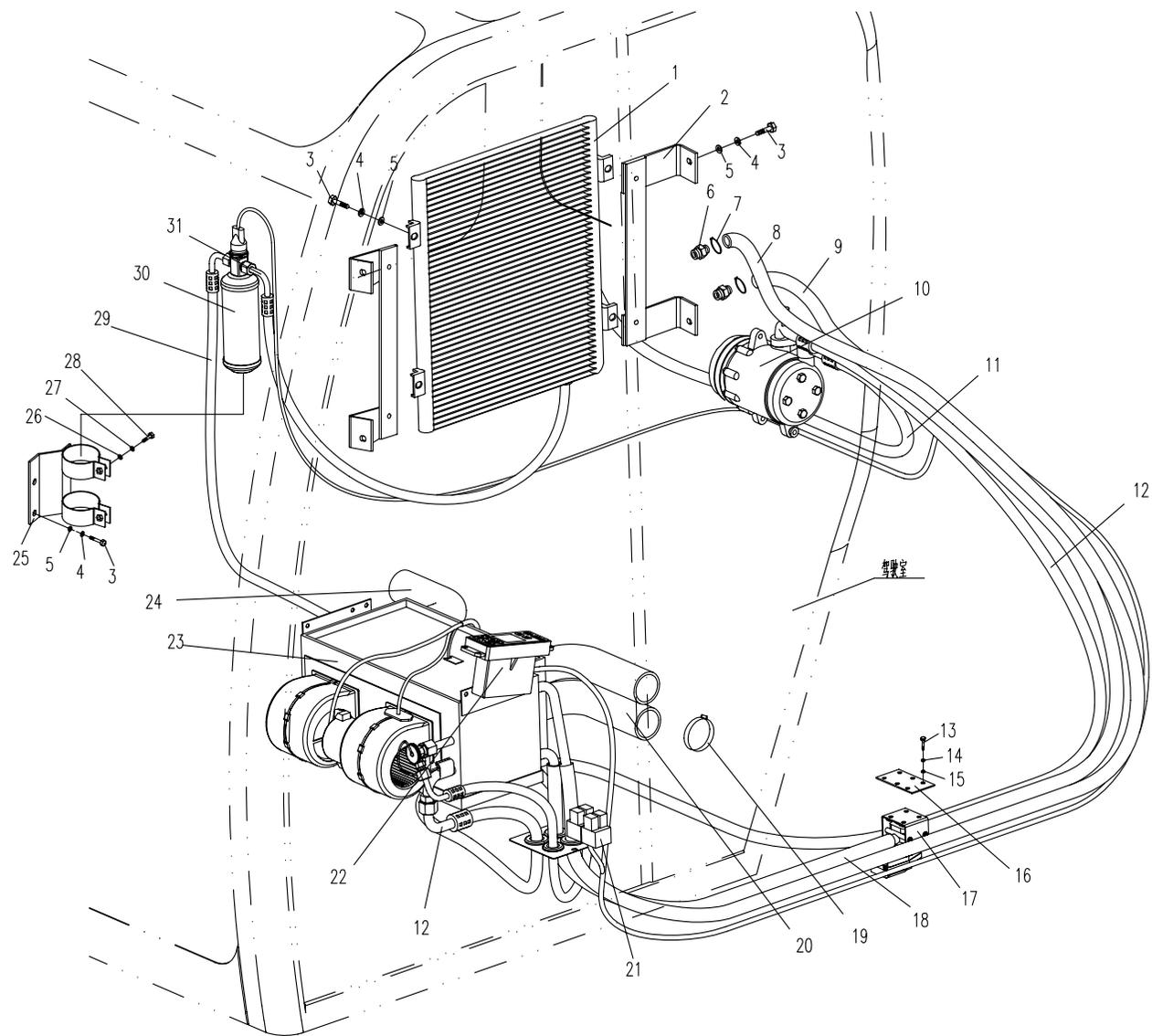
08.1.1 空调系统 (适用858机型) AIR-CONDITION SYSTEM (APPLY TO 858 TYPE)
