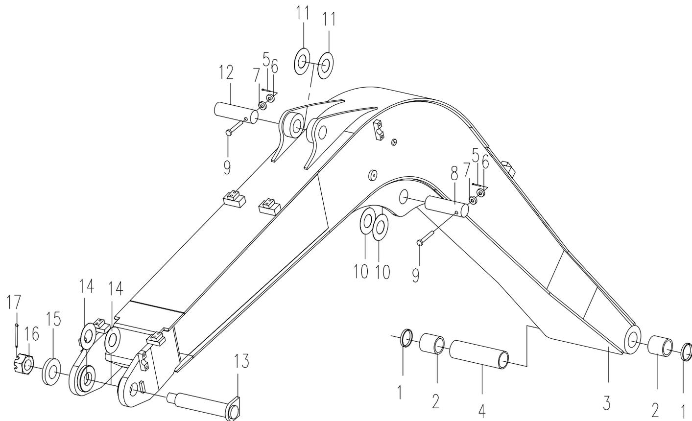
04.2.1 工作装置 2(适用858,858A机型) WORKING EQUIPMENT 2 (APPLY TO 858,858A TYPE)
