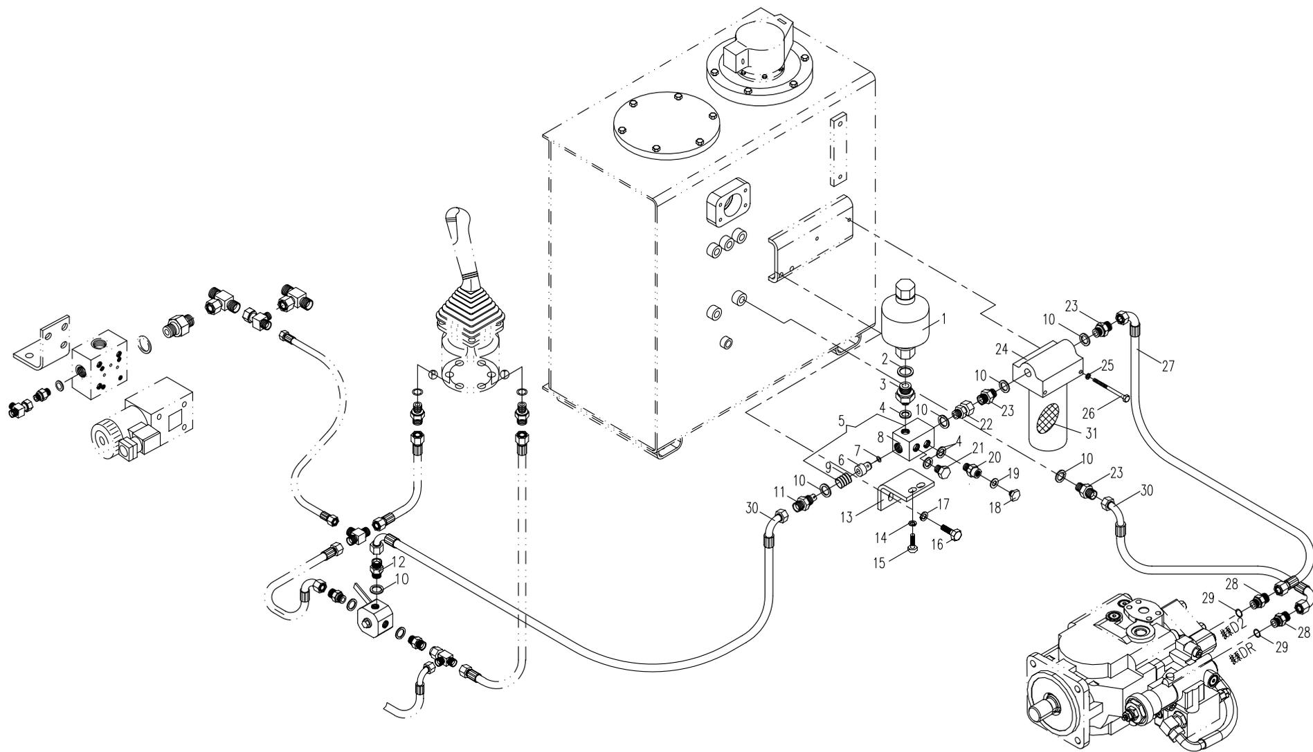
85.1.1 先导部分的液压系统1 (适用858,858A机型) HYDRAULIC SYSTEM FOR PILOT PART 1 (APPLY TO 858,858A TYPE)
