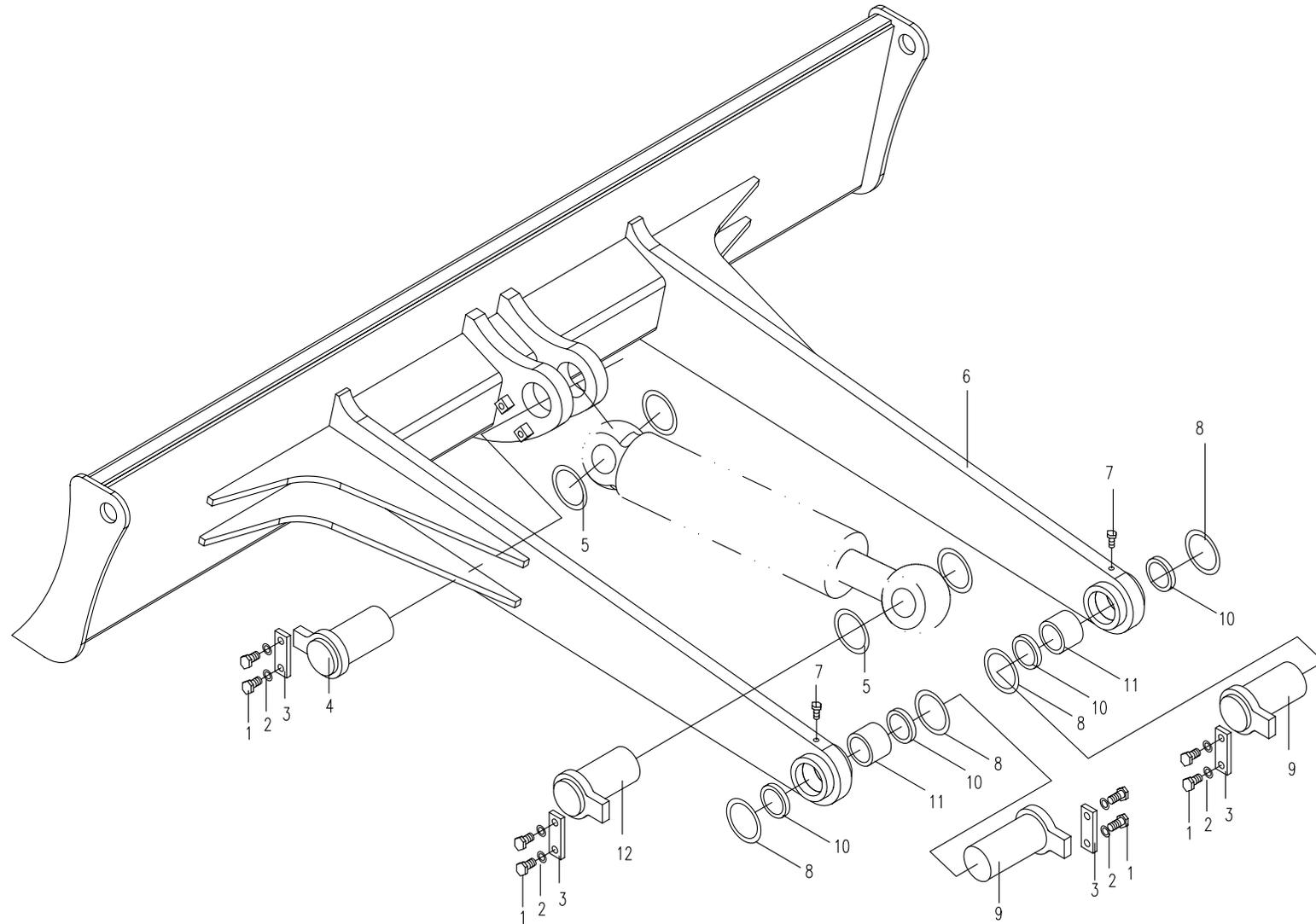
04.1.1 工作装置 1 (适用858, 858A机型) WORKING EQUIPMENT 1 ( APPLY TO 858,858A TYPE)
