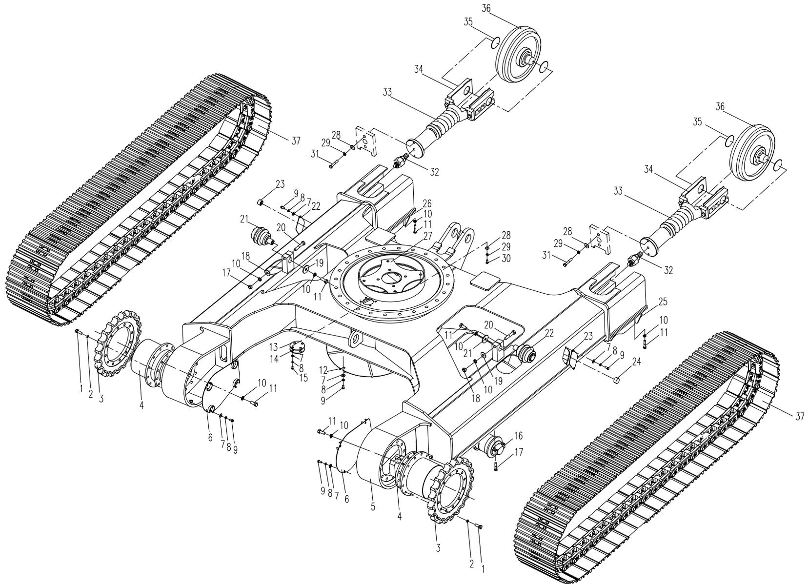
01.1.1 底盘总成(适用858, 858A机型) CHASSIS ASSEMBLY (APPLY TO 858,858A TYPE)
