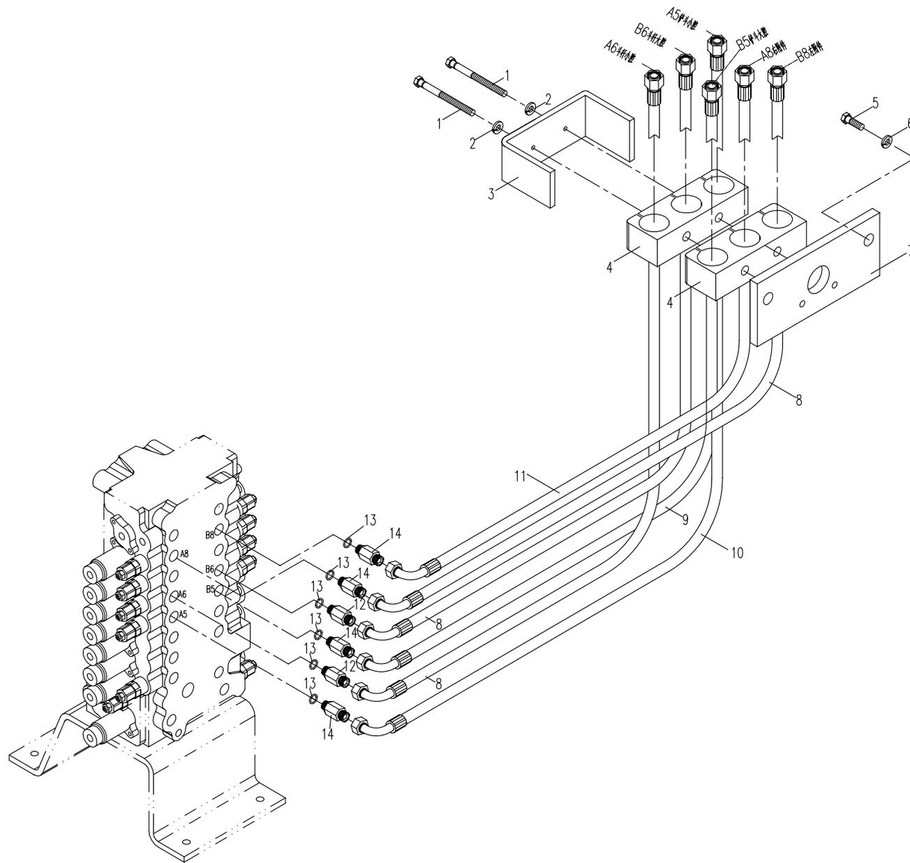
75.1.1 底盘部分的液压系统1 (适用858,858A机型) HYDRAULIC SYSTEM FOR CHASSIS 1 (APPLY TO 858, 858A TYPE)
