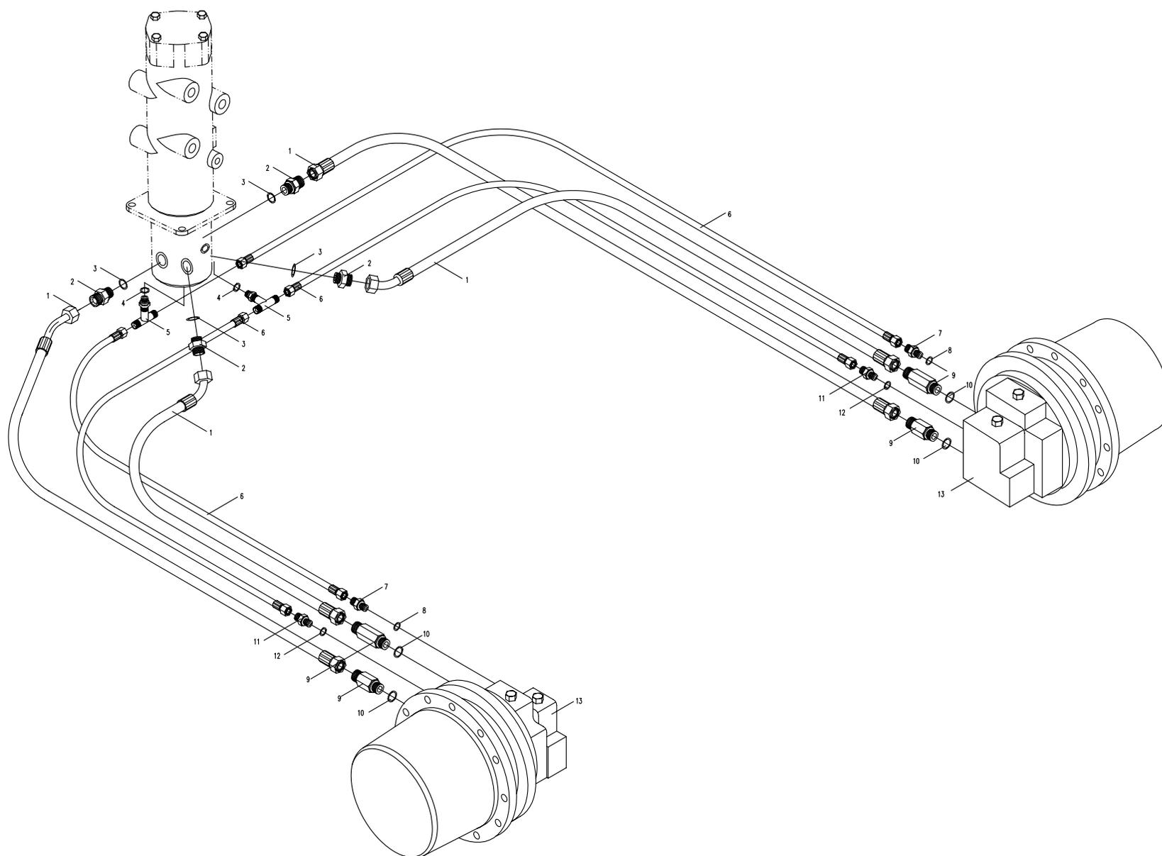
75.2.1 底盘部分的液压系统2 (适用858,858A机型) HYDRAULIC SYSTEM FOR CHASSIS 2 (APPLY TO 858, 858A TYPE)
