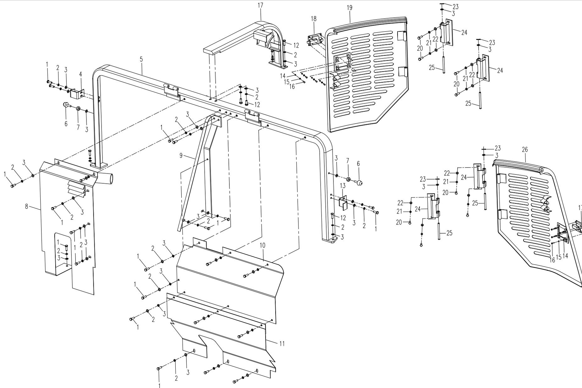
09.2.1 單框总成2 (适用858, 858A类型) COVER ASSEMBLY 2 (APPLY TO 858, 858A TYPE )
