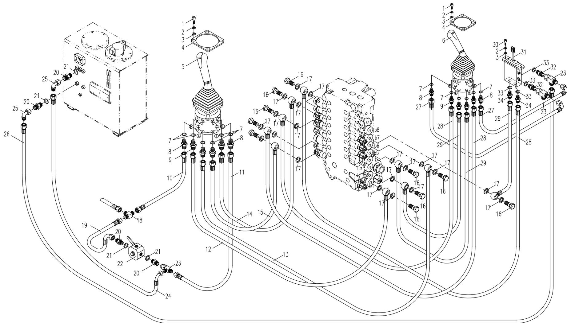
85.2.1 先导部分的液压系统2 (适用858,858A机型) HYDRAULIC SYSTEM FOR PILOT PART 2 (APPLY TO 858,858A TYPE)
