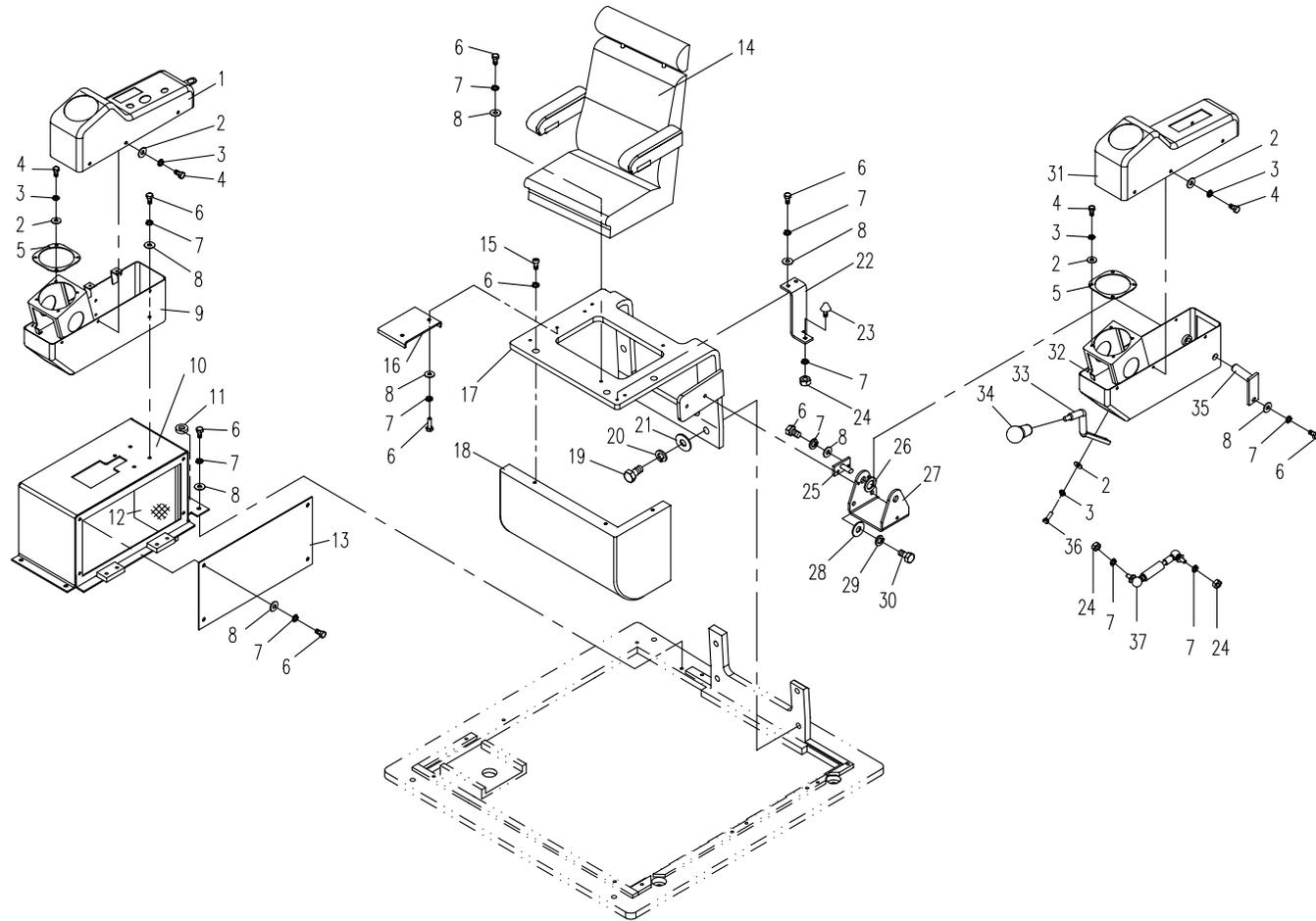
06.1.1 操纵机构1 (适用858,858A机型) CONTROL FRAMEWORK 1 (APPLY TO 858,858A TYPE)
