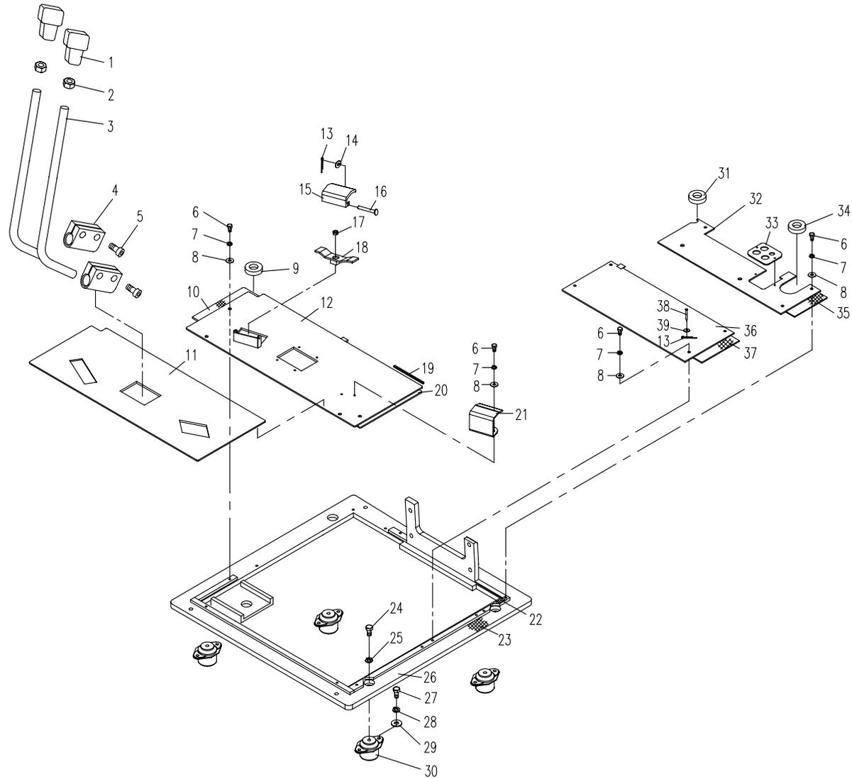
06.1.2 操纵机构2 (适用858,858A机型) CONTROL FRAMEWORK 2 (APPLY TO 858,858A TYPE)
