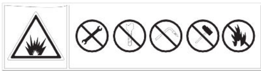
25) Do not split, drill, cut or impact the Accumulators, air spring pressure device and keep them away from open fire and heat.
